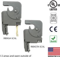
Example: With a current of 10 amps set as the threshold and a 15% differential, sensor contact will be closed between 8.5 amps and 11.5 amps and open outside of this range. A small amount of hysteresis is provided to prevent dithering near the differential limits.
